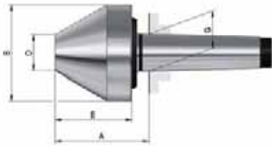
A06 Revolving centering taper, cone truncated, 60°
