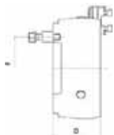
A08 ISO 702-3 (DIN 55027), with studs and locknuts
