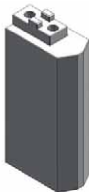
Jaw blank - aluminium (including fixing screws)
